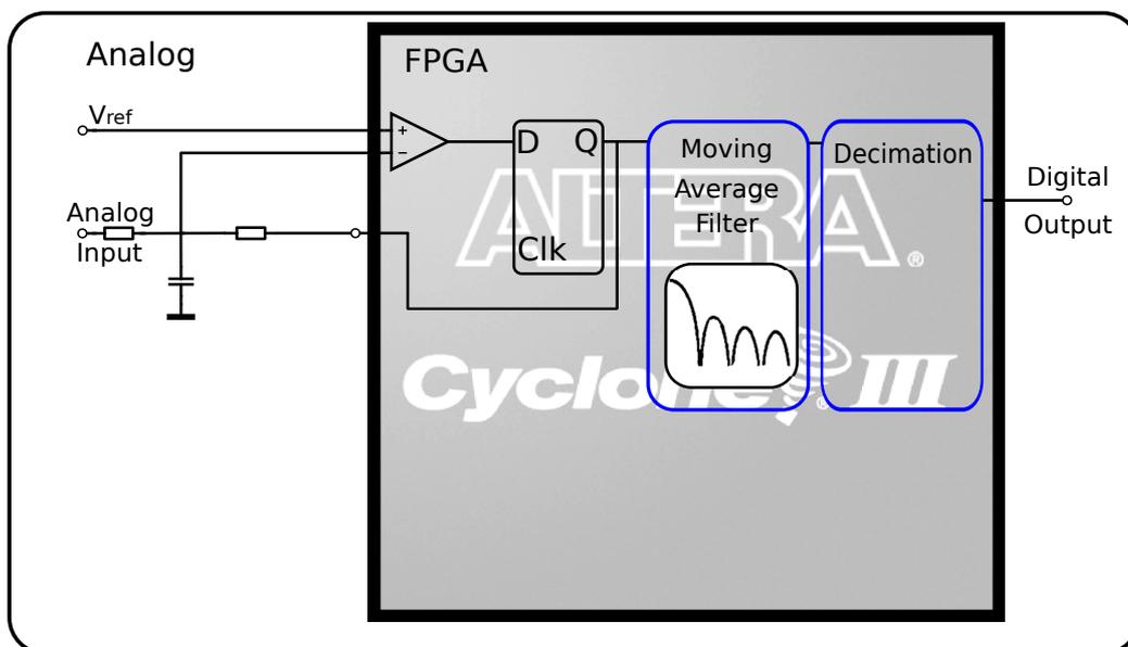
Figure 5: Principle of the Delta Sigma Modulator using LVDS receivers
