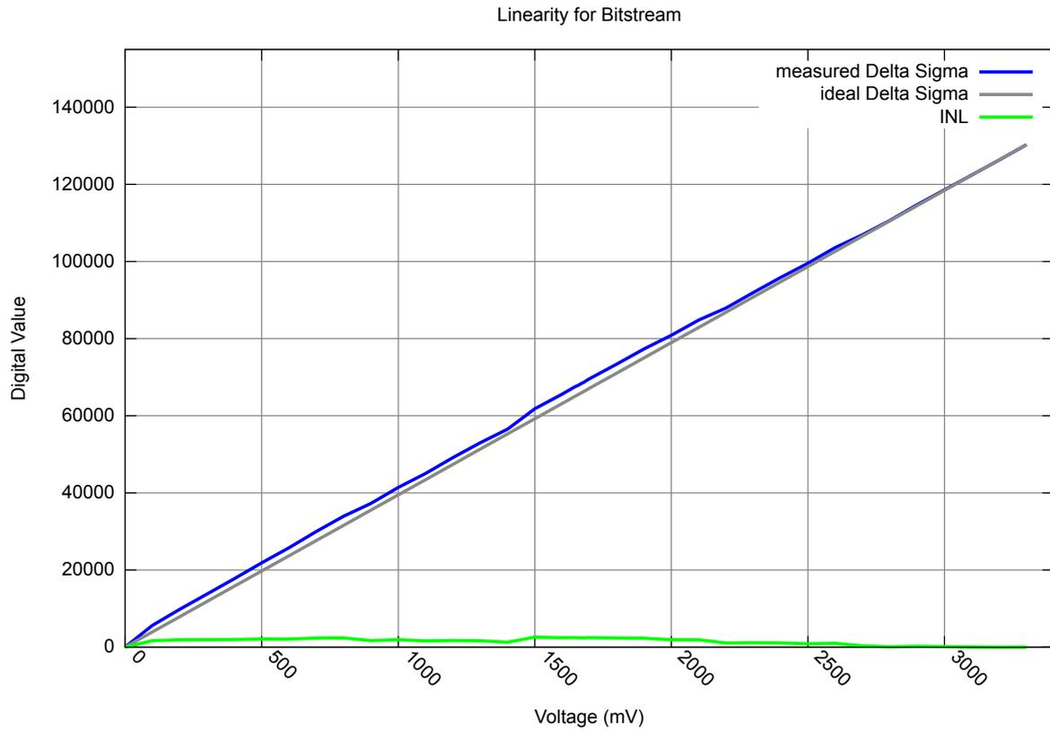
Figure 7: Plot of Linearity Voltage over digital Value
