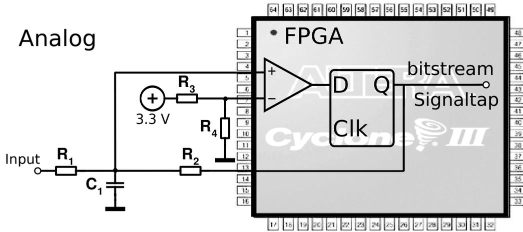
Figure 6: Schematic
