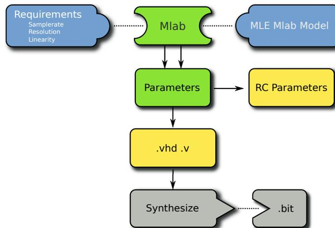
Figure 3: Design Flow for a Delta Sigma ADC Parameterization
