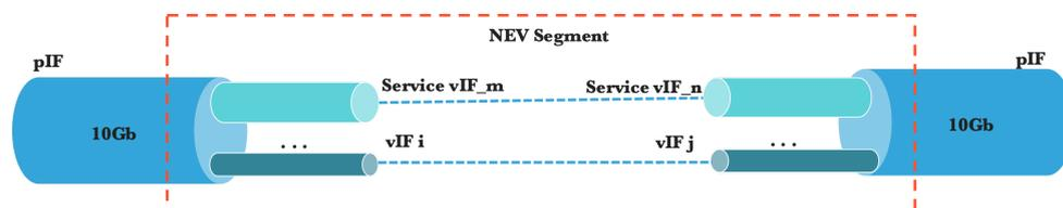
As a result, a physical network interface (pIF) can carry many so-called NEV Service Virtual Interfaces (sIF). Algotblu developed a centralized PTS(Primary Telco Services) OAM system to control and to manage this virtualization, including dynamic adjustments of bandwidth, on a network segment by network segment basis.
