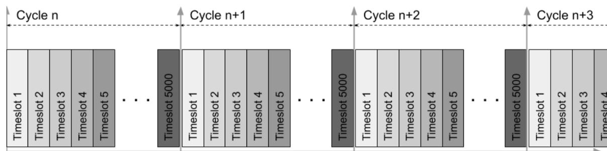
Another way to represent this can be a “wheel” with 5000 Timeslots where each sIF can occupy zero, or more, Timeslots: The following figure visualizes how different sIF can be run using NEV:
