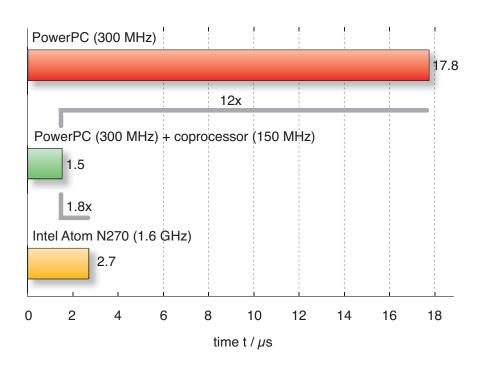
Figure 2 – The hardware-accelerated system (green bar, center) ran faster than a standalone PowerPC or an Atom processor.
