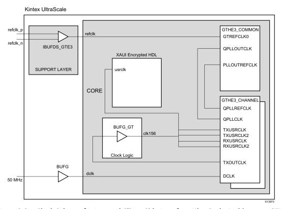
Figure 6-6: Clock Scheme for Internal Client-Side Interface UltraScale Architecture GTH Transceiver Shared Logic in Example Design
