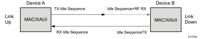
Figure C-5: Device A Receives Idle Sequence
