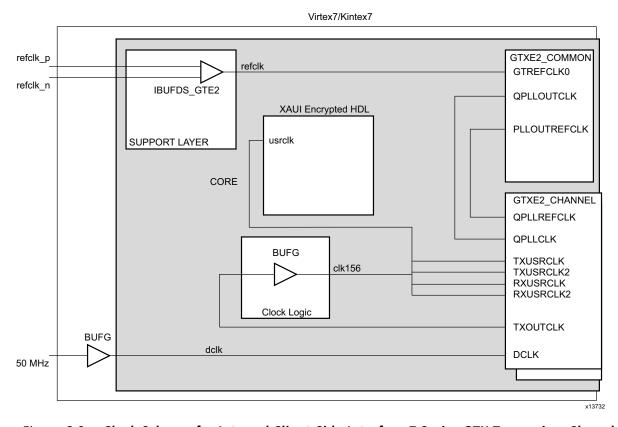
Figure 6-9: Clock Scheme for Internal Client-Side Interface 7 Series GTX Transceiver Shared Logic in Core
