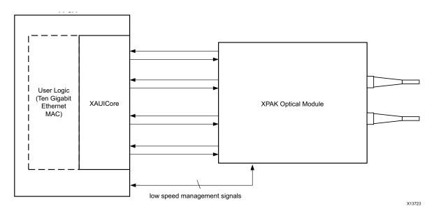
Figure 4-1: Connecting XAUI to an Optical Module
