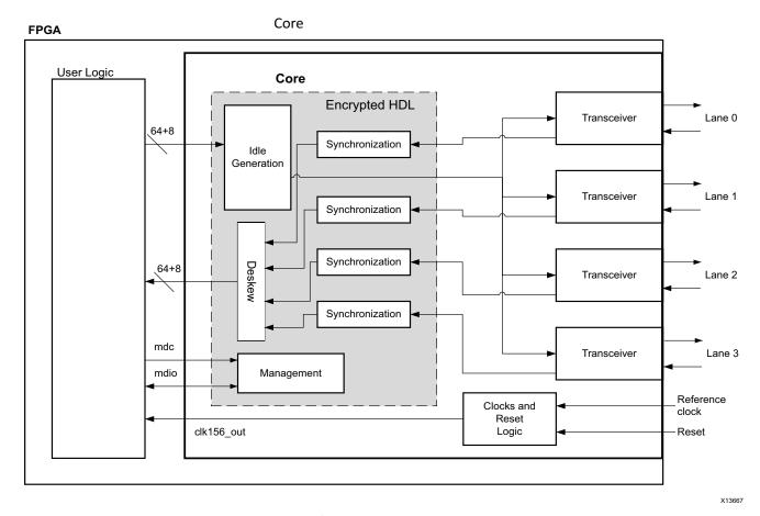
Figure 1-1: Architecture of the XAUI IP Core with Client-Side User Logic
