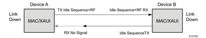
Figure C-4: Device B Powers Up and Resets
