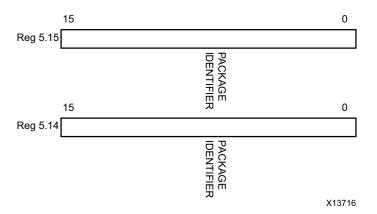
Figure 5-36: DTE XS Package Identifier Registers
