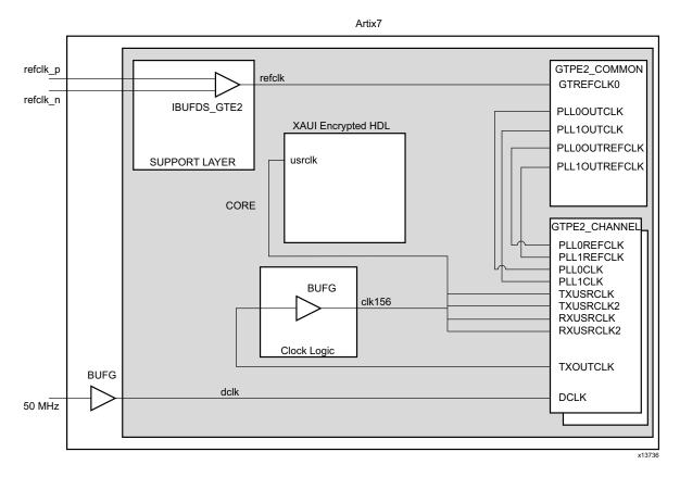
Figure 6-7: Clock Scheme for Internal Client-Side Interface 7 Series FPGA GTP Transceiver Shared Logic in Core
