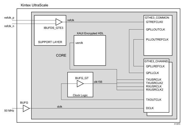
Figure 6-10: Clock Scheme for Internal Client-Side Interface UltraScale Architecture GTH
