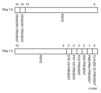
Figure 5-15: PMA/PMD Devices in Package Registers
