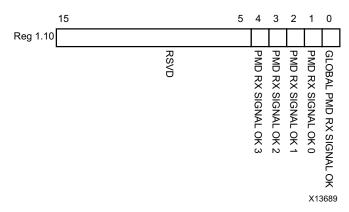
Figure 5-18: 10G PMD Signal Receive OK Register
