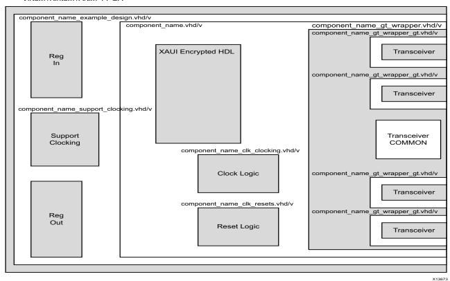
Figure 8-1: Example HDL Wrapper for XAUI with Shared Logic in the Example Design (7-Series FPGAs)
