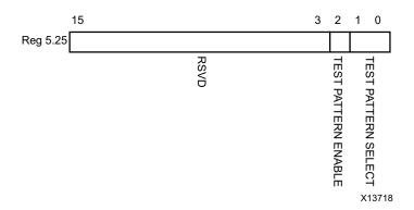
Figure 5-38: 10G DTE XGXS Test Control Register
