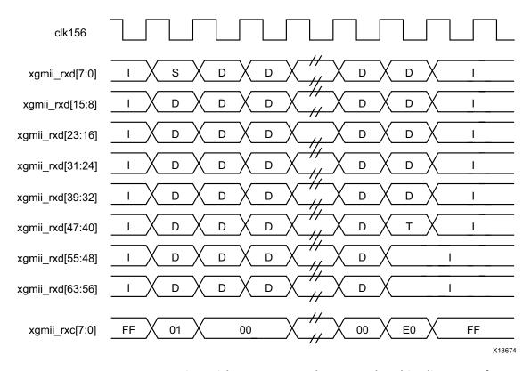
Figure 5-4: Frame Reception with Error Across the Internal 64-bit Client Interface
