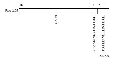
Figure 5-29: Test Control Register
