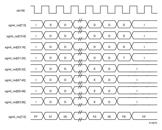
Figure 5-3: Frame Reception Across the Internal 64-bit Client Interface
