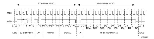
Figure 5-10: MDIO Read-and-increment Transaction
