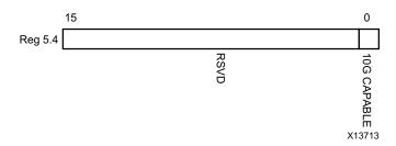
Figure 5-33: DTE XS Speed Ability Register
