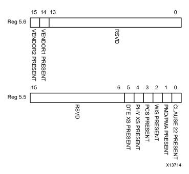
Figure 5-34: DTE XS Devices in Package Register
