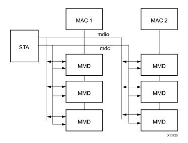
Figure 5-5: A Typical MDIO-Managed System
