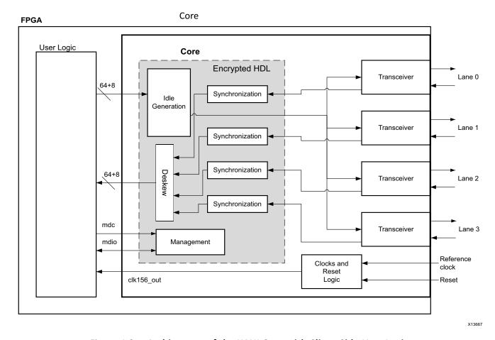
Figure 4-3: Architecture of the XAUI Core with Client-Side User Logic
