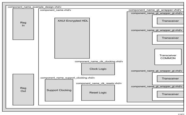
Figure 8-2: Example HDL Wrapper for XAUI with Shared Logic in Core (7-Series FPGAs)
