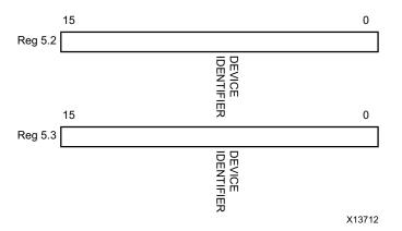
Figure 5-32: DTE XS Device Identifier Registers
