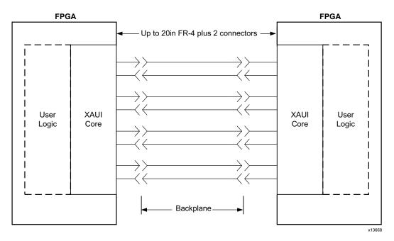
Figure 1-3: Typical Backplane Application for XAUI
