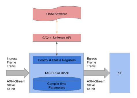
Via a software API, bandwidth, traffic priority, traffic burstiness, etc. can be controlled by assigning certain Service Interfaces to timeslots in the Traffic Shaper. Short cycle times, enabled by network protocol processing in PL, keeps processing latencies short and deterministic.
