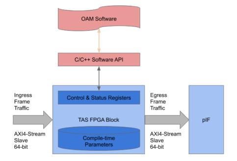
Via a software API, bandwidth, traffic priority, traffic burstiness, etc. can be controlled by assigning certain Service Interfaces to timeslots in the Traffic Shaper. Short cycle times, enabled by network protocol processing in PL, keep processing latencies short and deterministic.
