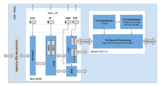
Since the TCP/IP stack and the TLS 1.3 security protocol – including importantly both key exchange and key management – are both executed entirely in hardware, the joint solution has both scalable high-speed performance and minimizes attack surface, especially when compared to a software-based approach. The FPGA hereby utilizes the hardware Root of Trust, best suited for applications like critical communication in defense, space technology, and energy production and distribution .
