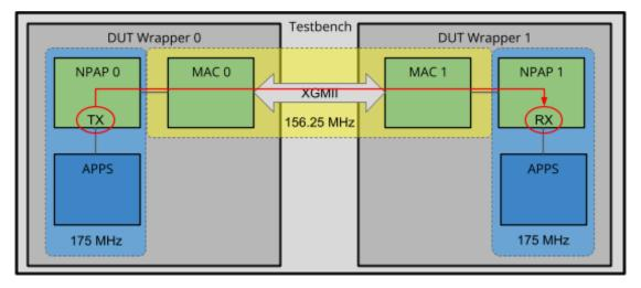
Obviously, increasing the NPAP clock frequency will reduce RTT latency for asynchronous NPAP subsystems.
