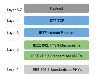
The outcome is a deterministic and reliable network protocol, which makes TCP/IP over TSN a very good candidate for all networking where IT (Information Technology) and OT (Operations Technology) converge, or in Systems-of-Systems backbones. TSN itself is quickly evolving so please contact us for more information!
