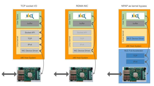
NPAP can operate in a similar way, where NPAP does all TCP/IP processing in dedicated ASIC / FPGA logic and then a (Linux) device driver copies the payload data between user space memory and NPAP.
