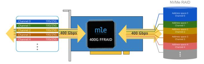
Now, you can transfer bulky data from multiple sensors to a RAID of NVMe SSDs at speeds up to 400 Gbps. MLE's NVMe Fast FPGA RAID implements a channel-based architecture, supports data-in-motion pre- and post-processing and is highly scalable with regards to bandwidth and recording capacity. Multiple systems can further be cascaded via high-accuracy IEEE time-synchronization for faster or deeper recording.
