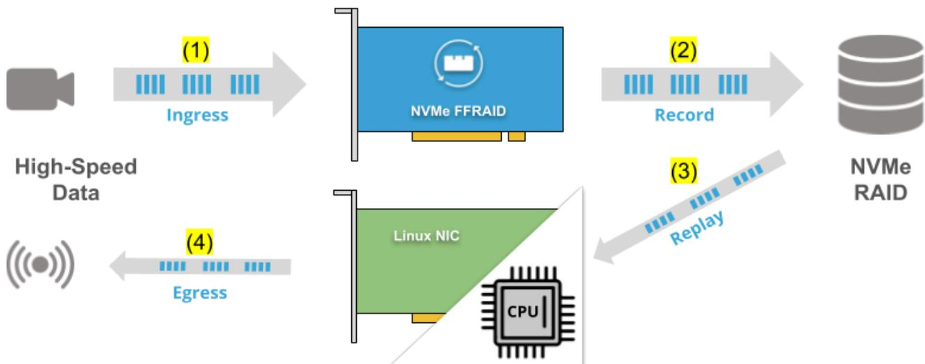
Ingress data (1) is recorded at high-speed using MLE NVMe FFRAID acceleration (2). Once recording is done the MLE NVMe FFRAID releases the SSD RAID and Linux opens this as an MDRAID. Then data can be replayed via Linux (3), typically at lower speeds, and, for example sent out via a Linux network connection (4).
