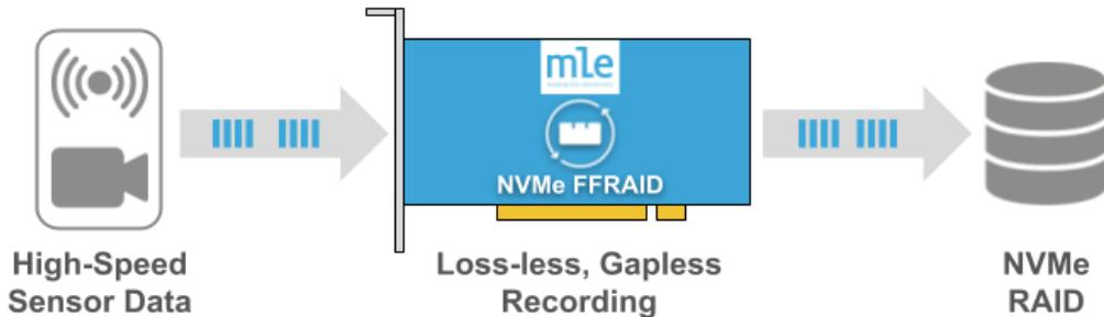
Ingress data from the high-speed sensors are transferred and recorded at-speed and as-is onto the NVMe Fast FPGA RAID.
