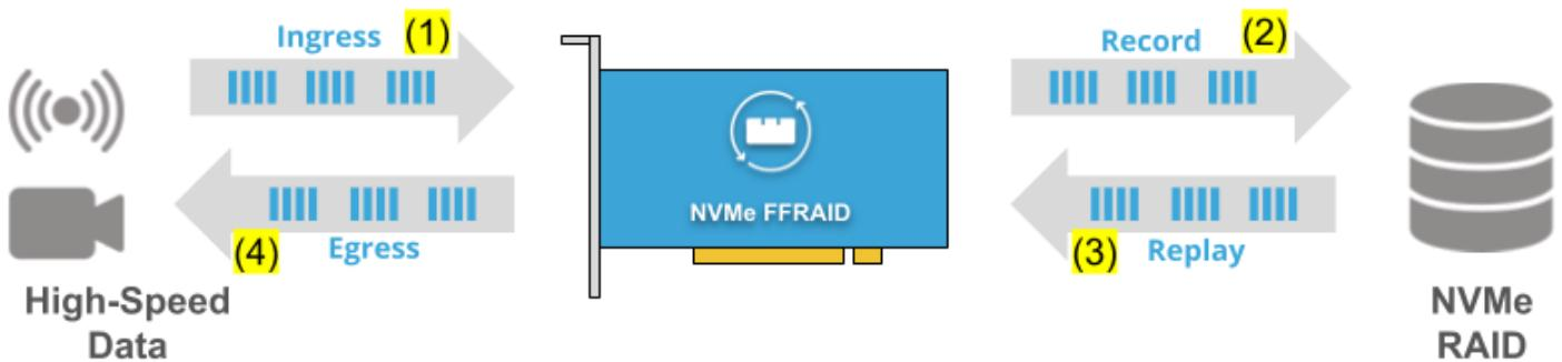
Ingress data (1) is recorded at high-speed using MLE NVMe FFRAID acceleration (2). Once recording is done, then data can be replayed via MLE NVMe FFRAID (3) and be streamed-out at high data rates (4). Because you operate the NVMe SSDs purely in sequential read (ex-or write), this features best performance.
