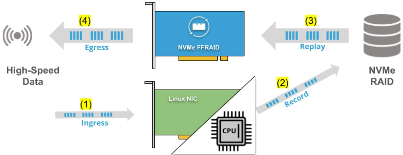
Ingress data (1) comes in via a Linux NIC, or any other Linux userspace software, for example, and is recorded onto a Linux MDRAID (2). Once recording is done, Linux releases the SSD RAID and the MLE NVMe FFRAID then opens it. Then data can be replayed via MLE NVMe FFRAID (3) and be streamed-out at high data rates (4).
