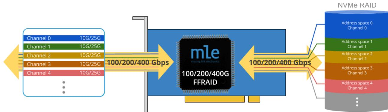
Now, you can transfer bulky data from multiple sensors to a Redundant Array of Inexpensive NVMe SSDs at speeds up to 400 Gbps. MLE NVMe FFRAID implements a channel-based architecture, supports data-in-motion pre- and post-processing and is highly scalable with regards to bandwidth and recording capacity. Multiple systems can further be cascaded via IEEE 1588-2019 (HA) Precision Time Synchronization (PTP) for faster and/or deeper recording.
