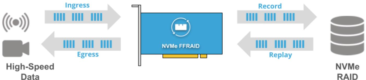
Ingress data is recorded at high-speed using MLE NVMe FFRAID acceleration. At the same time, while recording, data is replayed from the MLE NVMe FFRAID and be streamed-out at high data rates. Because typical NVMe SSDs deliver less performance when writes happen parallel to reads, you will experience less performance in this mode.
