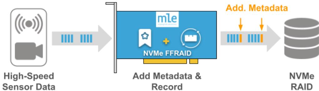
Ingress data can be analyzed on-the-fly to generate indexing information for later search, for example. This metadata is then recorded along with the ingress data. Metadata can, for example, be: Hardware timestamps, regions-of-interest, search indexes.
