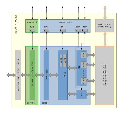
The datapath goes horizontally, with ingress and egress 10/25/50/100 Gigabit Ethernet on the left into/out of dedicated FPGA/ASIC hardware blocks:
