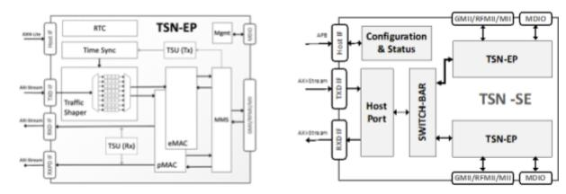
Real-time configuration needs little compute performance and runs in software either on the Host CPU (which can be PCIe-connected) or SoC-style on an embedded CPU. Unlike in a typical CPU/software implementation where the "upstream" port of the TSN Switched Endpoint connects to a DMA engine, in a TCP-TSN-Core this is connected to
