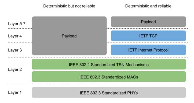
The outcome is a deterministic and reliable network protocol, which makes TCP/IP over TSN a very good candidate for all networking where IT (Information Technology) and OT (Operations Technology) converge, or in Systems-of-Systems backbones such as Automotive Zone Architectures.
