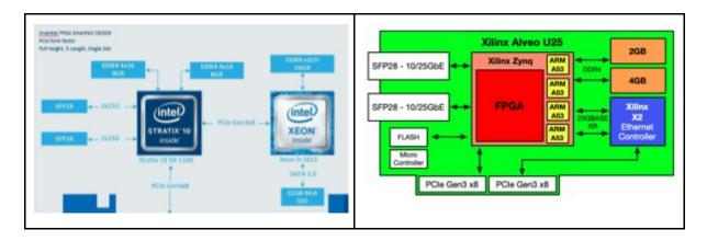
When using such FPGA-Based SmartNICs, network protocol processing can be performed on three stages using three different cores, as the following Figures shows:
