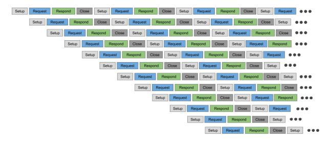
Implementing such a pipelining approach is facilitated by yet another advantage of TCP-TSN-Cores: Opening, processing and closing takes significantly less time compared to software, if the network is fast, and if the counterpart is also fast. Best is to have similar TCP-TSN-Cores on either side of the TCP connection.
